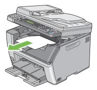
5 Remove any paper in the priority sheet inserter (PSI) or multipurpose feeder (MPF). Keep the paper wrapped and away from humidity and dirt.
