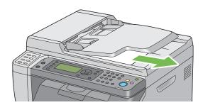
4 Remove any paper in the center output tray if there is. Close the output tray extension if it is extended.
