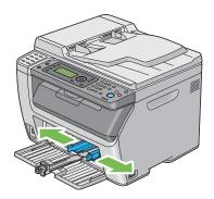
6 Before loading the print media, flex the sheets back and forth, and then fan them. Straighten the edges of the stack on a level surface.
