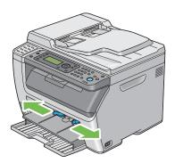
4 Before loading the print media, flex the sheets back and forth, and then fan them. Straighten the edges of the stack on a level surface.
